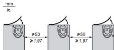
By removing the protective blanking cover from the top of the drive, the degree of protection for the drive becomes IP21. The protective blanking cover may vary according to the drive model, see opposite.
