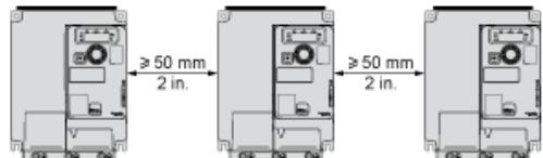
Only Possible at Ambient Temperature Less or Equal to 50 °C (122 °F)
