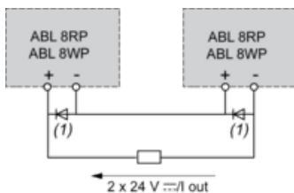
(1) Two Shottky diodes  $I_{min} = \text{power supply } I_{in}$  and  $V_{min} = 50 \text{ V}$
