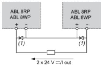
(1) Two Shottky diodes  $I_{min} = \text{power supply In}$  and  $V_{min} = 50 \text{ V}$
