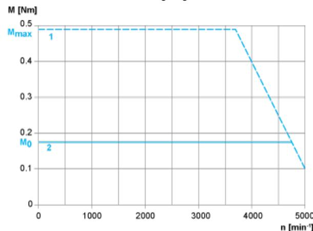
Torque/Speed Curves with 230 V Single/Three Phase Supply Voltage
