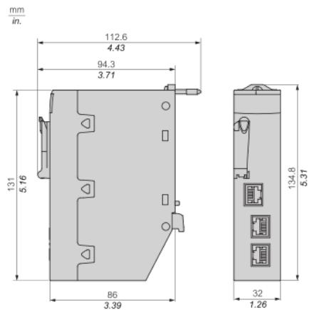
Module mounted on rack
