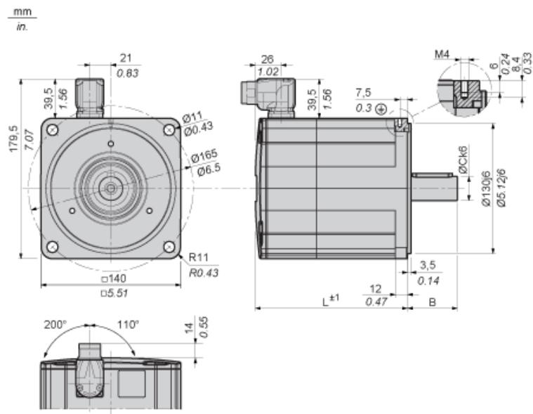
Parallel Key According to DIN 6885 A
