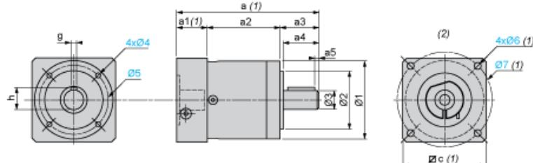
(1) Dimensions a, a1, c, Ø6 and Ø7 depend on the planetary gearbox/servo motor combination
