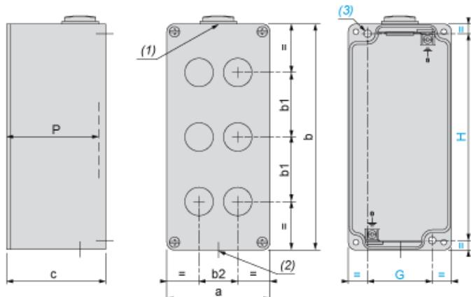
(1) : 1 hole, with blanking plug (protrusion 6 mm/0.24 in.), for cable gland ISO M20 x 1.5
