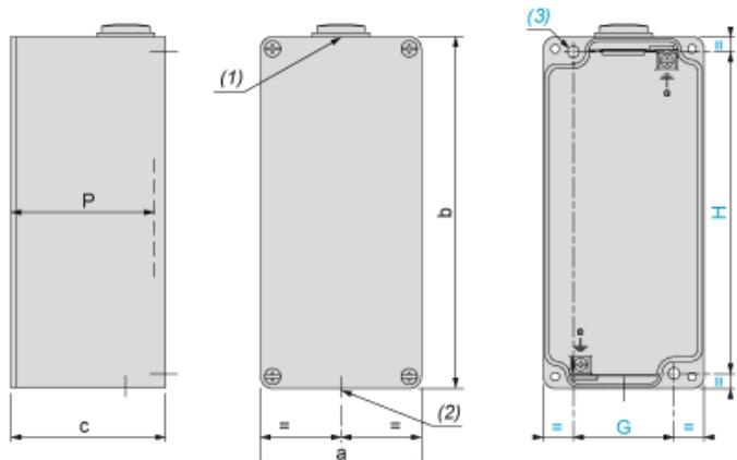
(1) : 1 hole, with blanking plug (protrusion 6 mm/0.24 in.), for cable gland ISO M25 x 1.5
