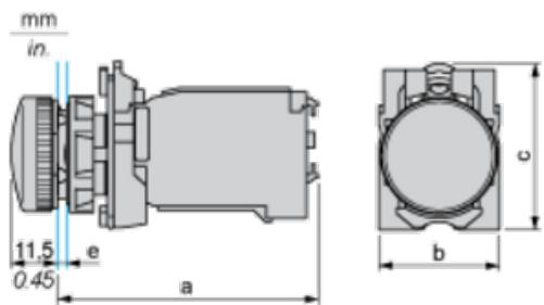
e: clamping thickness: 1 mm to 6 mm / 0.04 in. to 0.24 in.
