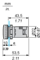
e Support panel thickness: 1 to 6 mm/0.4 to 0.24 in. (metal), 2 to 6 mm/0.8 to 0.24 in. (plastic).
