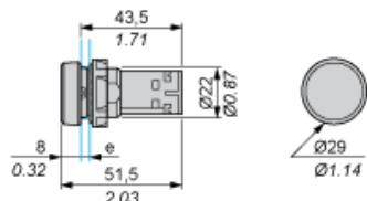
e Support panel thickness: 1 to 6 mm/0.4 to 0.24 in. (metal), 2 to 6 mm/0.8 to 0.24 in. (plastic).
