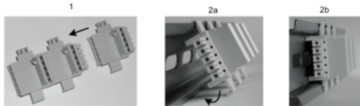
1 : Connect as much Backplane Connector as module to be install.
