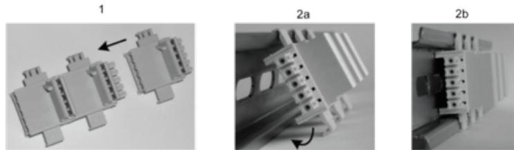
1 : Connect as much Backplane Connector as module to be install.
