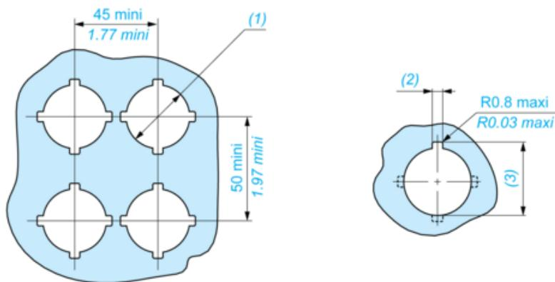
(1)  $\varnothing 30.75 \text{ mm} \pm 0.25$  recommended ( $\varnothing 30.5 \text{ mm} \text{ }_0^{+0.5}$ ) /  $\varnothing 1.21 \text{ in.} \pm 0.0098$  recommended ( $\varnothing 1.21 \text{ in.} \text{ }_0^{+0.0196}$ )
