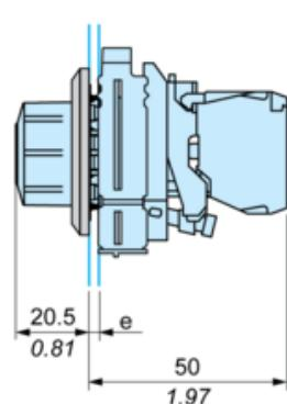
e : clamping thickness: 1 to 4.35 mm / 0.04 to 0.17 in.
