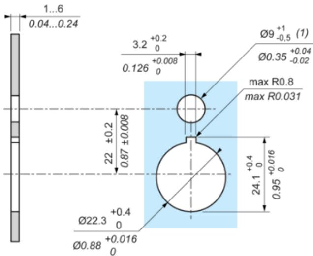
(1) : For IP X9 applications, the max recommendation dimension of hole is Ø9 mm/Ø0.35 in.
