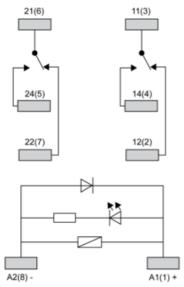
NOTE: For DC input , A1 have to be + , otherwise it would short circuit from protection module
