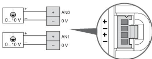
The (-) poles are connected internally.
