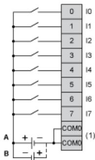
(1) The COM0 terminals are connected internally.
