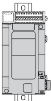
NOTE: Expansion modules must be mounted above the logic controller.
