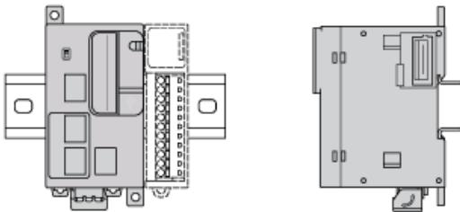
NOTE: Keep adequate spacing for proper ventilation and to maintain an ambient temperature between -10°C (14°F) and 55°C (131°F).
