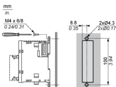
Digital Relay Output Module (16-channel)
